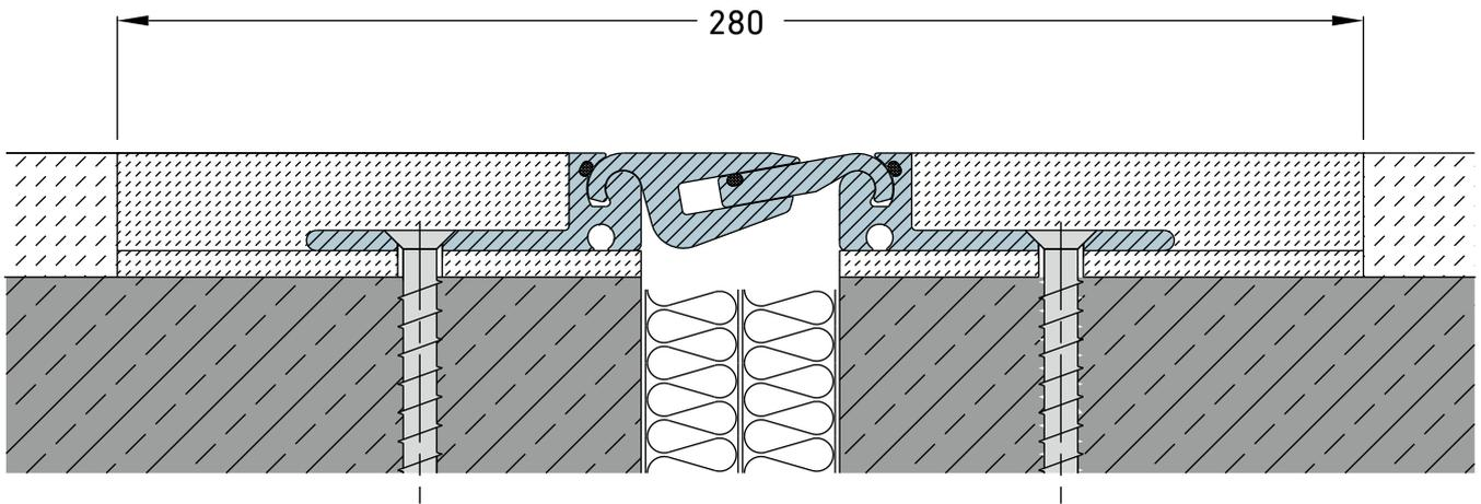
MIGUTRANS expansion joint construction, e.g. in conjunction with hard-aggregate floor screed, magnesite screed: FSX 75/22
