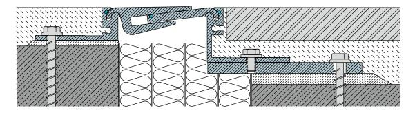
MIGUTRANS expansion joint construction with one-sided carry-over
