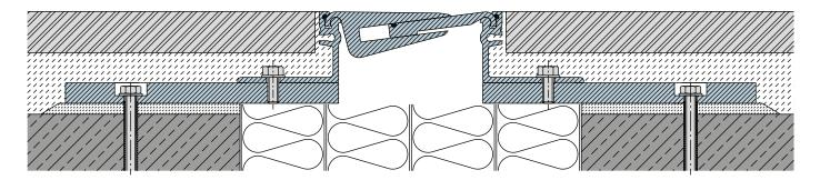
MIGUTRANS expansion joint construction with factory-supplied aluminium plates for extremely wide construction joints
