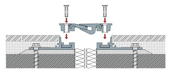
MIGUTRANS expansion joint construction FSRX with visible part that is exchangeable
