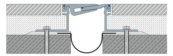
MIGUTRANS expansion joint construction with MIGUFOL tape
